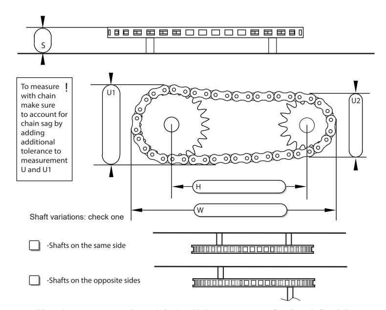
Additional measurements may be needed to be added to measurement A if you have shafts or hubs that extend past the sprockets. Other options may be available for your machine, please call to see what your best option is.
