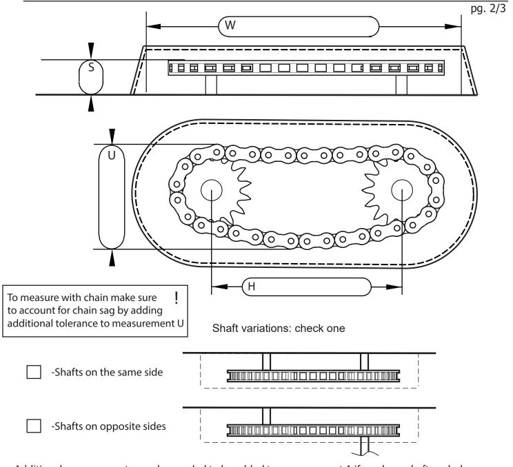
Additional measurements may be needed to be added to measurement A if you have shafts or hubs that extend past the sprockets.
