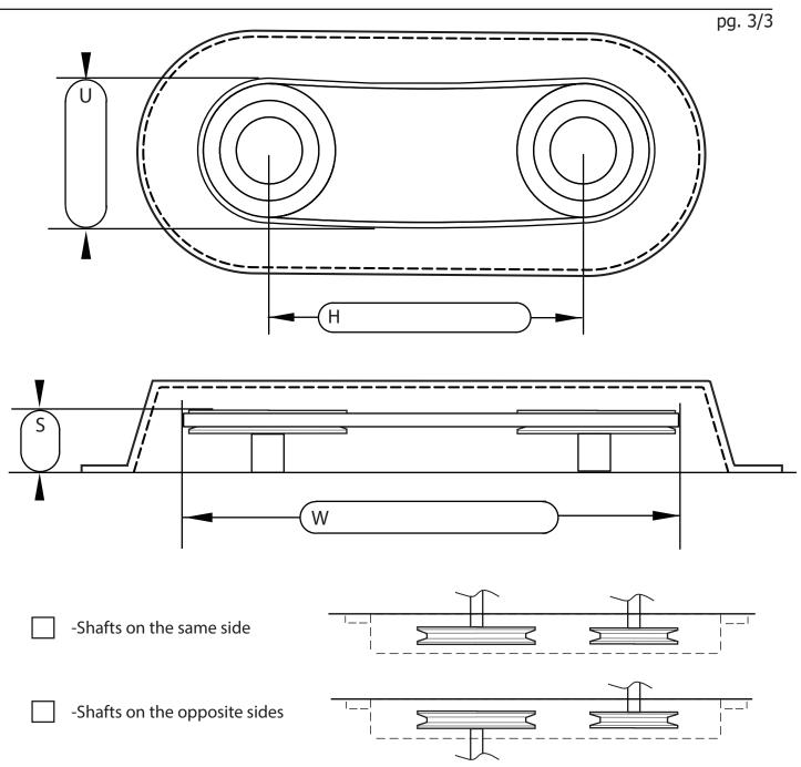
Additional measurements may be needed to be added to measurement A if you have shafts or hubs that extend past the sheaves.
