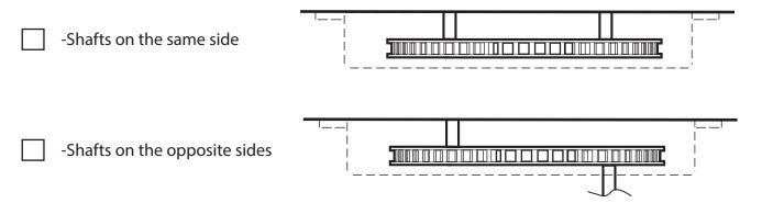
Additional measurements may be needed to be added to measurement A if you have shafts or hubs that extend past the sprockets.
