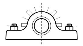
Note the position of any grease fittings by marking a box in the bearing drawing.
