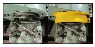
This before and after image shows an installed Split Round Guard point guarding the gap between a bushing (at bottom) and a gearbox (at top).
