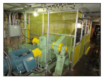
Using a "gotcha stick" gap measuring device, the distance to hazards directly behind the mesh was measured. The size of the openings in the mesh combined with the distance to the hazard locations required additional point quarding for several locations.
