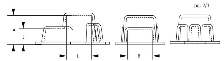
All measurements should be taken from the internal side of the guard to prevent unnecessary oversizing.
