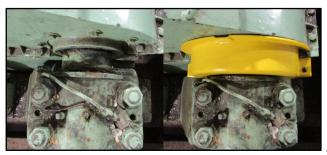
This before and after image shows an installed Split Round Guard point guarding the gap between a bushing (at bottom) and a gearbox (at top).
